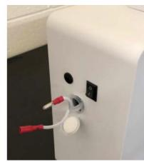
These wires supply power directly to the pump. The clock and controls will still work when this circuit is open.
