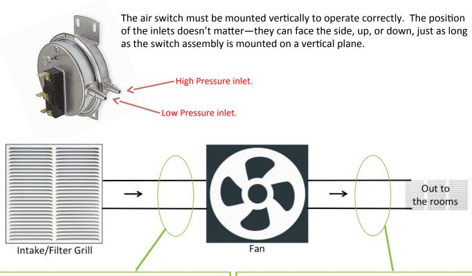
If the air switch is located between the air filter intake and the air fan, then you will need to set it up to detect LOW pressure when the fan comes on.
